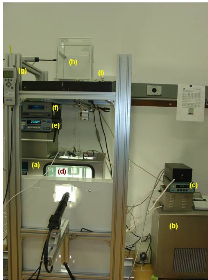
Figure 1. Hydrometer Calibration System of CENAM: (a) thermostatic bath, (b) external cooler, (c) external temperature controller, (d) glass vessel containing the reference liquid, (e) thermometer for temperature of liquid, (f) barometer, (g) thermo-hygrometer, (h) weighing instrument (balance), (i) mass standards.
